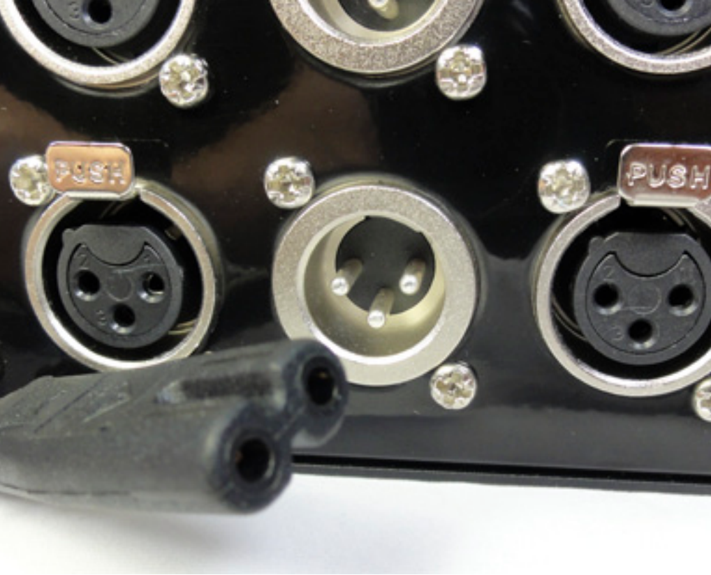
Plugging power cables into audio cables is a death sentence for any piece of audio equipment. Figure-eight cables coincidentally fit into XLR sockets, which happened in this case when someone was fumbling about on a darkened stage trying to plug a DJ console in. Don't make this mistake or it will be curtains for the audio device.
