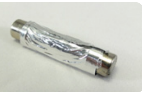
The industry standard approach to a blown fuse: 'wrap foil around it and jam it back in' is no approach at all. It's only a shortcut to equipment damage or personal injury. Avoid this technique like the plague.
