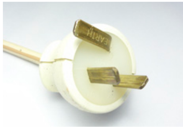
Never do this! Earth loop problems can always be solved in a way that's safe and leaves the mains earth pin intact. Apart from it being illegal, removing an earth pin to resolve an audio hum could kill you.
