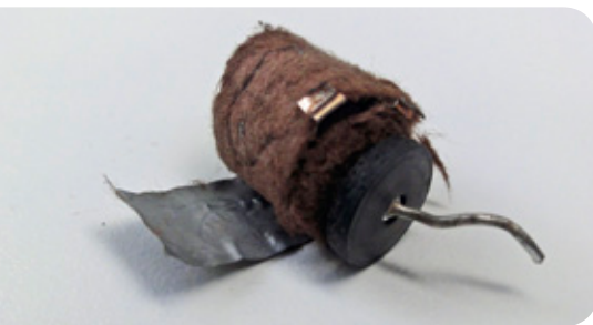
Roll out the barrel! This is what happens to an electrolytic capacitor when it's installed with reverse polarity, neatly revealing the rolled-up construction.
