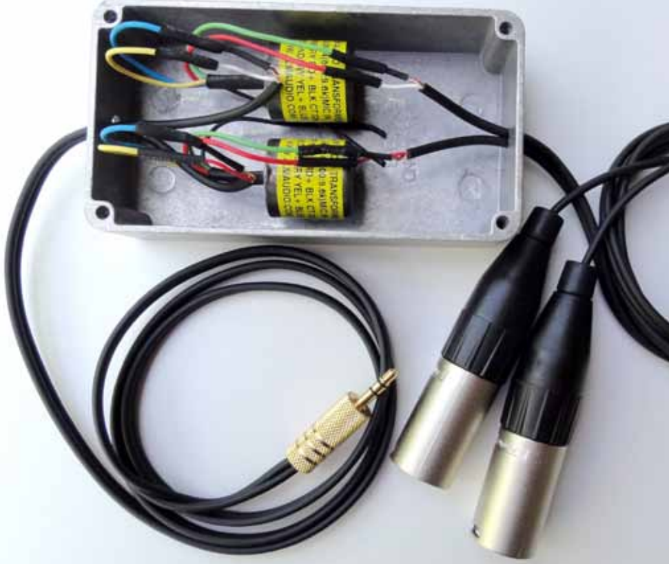
Wiring options: Above: a pair of JLM14 transformers adapt the 3.5mm plug to balanced XLRs; top right: the unbalanced TRS adapter cable option; and right: earth lifted XLR adapter cable.
