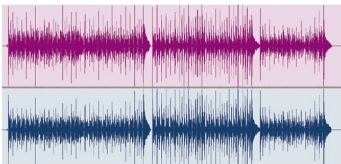
Unhealthy waveforms recorded too 'hot' into the DAW, causing distortion in the analogue path and digital clipping.
