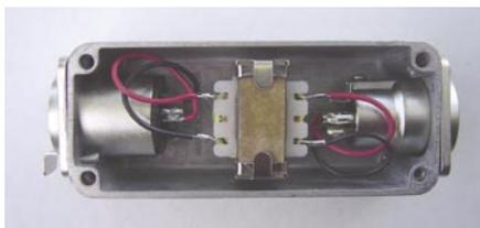
Above is an example of an audio isolation box where pins 2 and 3 of the XLRs connect to the transformer, while pin 1 (the ground pin) is left disconnected, thus separating the grounds. In this example an M0710 transformer from Altronics has been used. This is a surprisingly good line-level transformer. Its only shortcoming is its poor ability to drive low impedance loads. However, in a typical line level and line impedance situation (10 to 20kΩ) it can be just the ticket for ground isolation.
