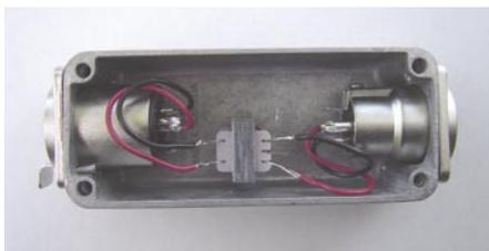
**An analogue microprocessor!** Here, the cheap little transformer – an M0222 – has been thrown into the same case as used in the previous isolation box example. Is this the smallest and cheapest effects box around?
